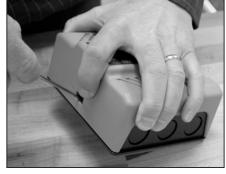
Turn box and repeat inserting screwdriver and pushin tab inward on opposite side, cover should release from base.
